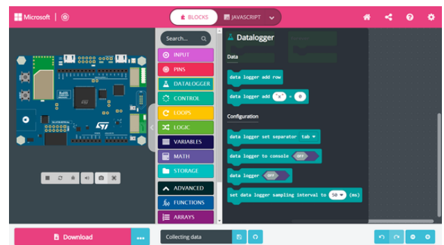
Datalogger and associated blocks
